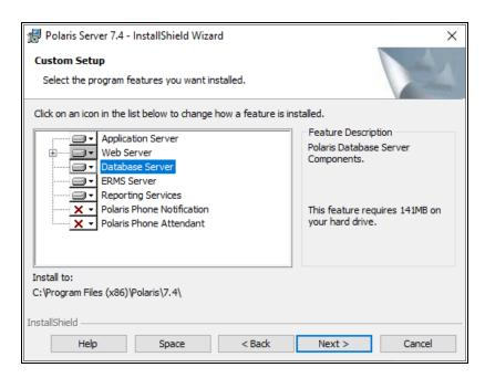
11. Select or deselect the server software to install on this computer by selecting a server name and selecting an option from the drop-down menu. For more
